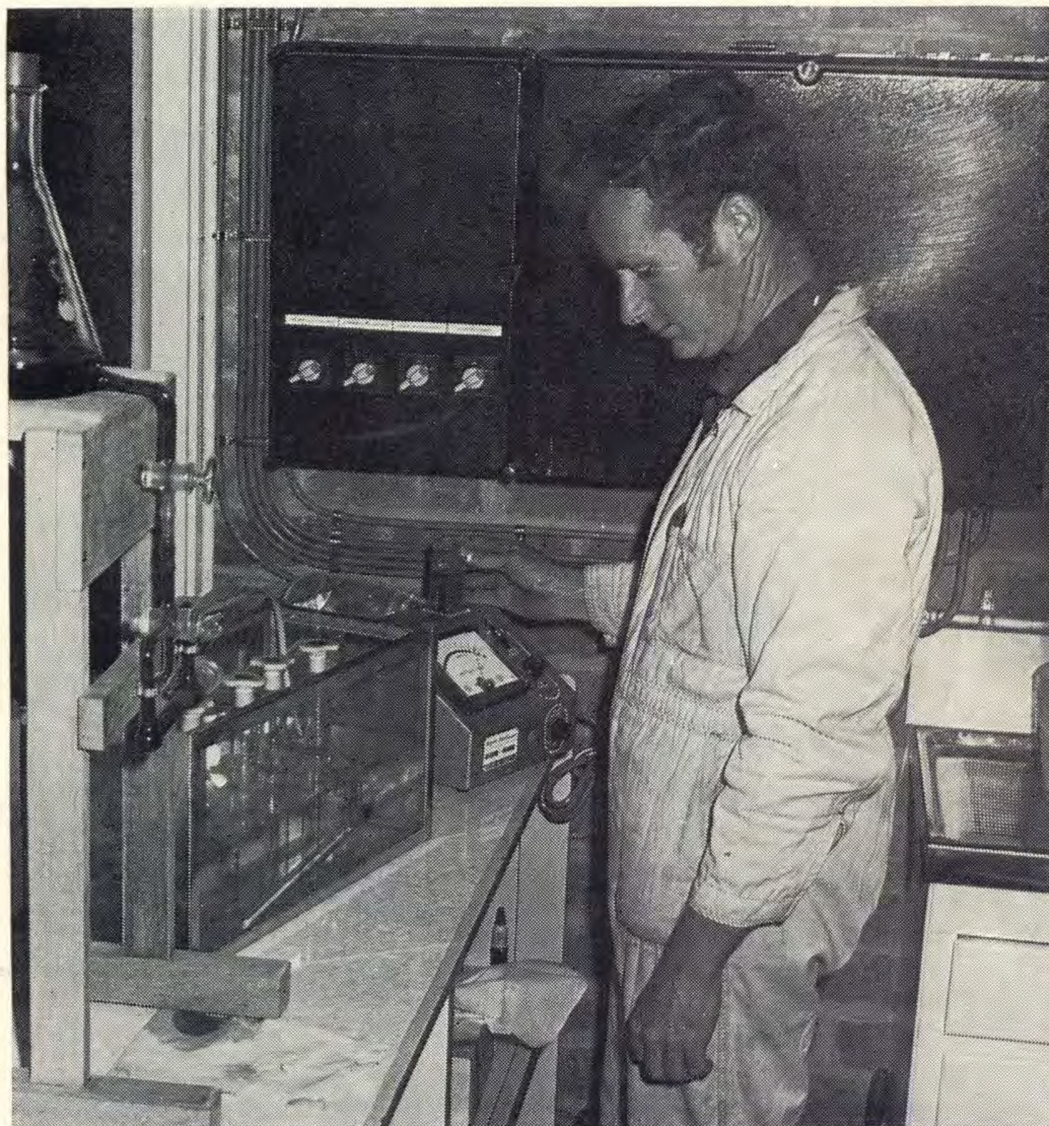
Reservoir Attendant Ken Patching tests a sample to ensure that the fluoride content is within the prescribed limit — 1 part in 1 million.
