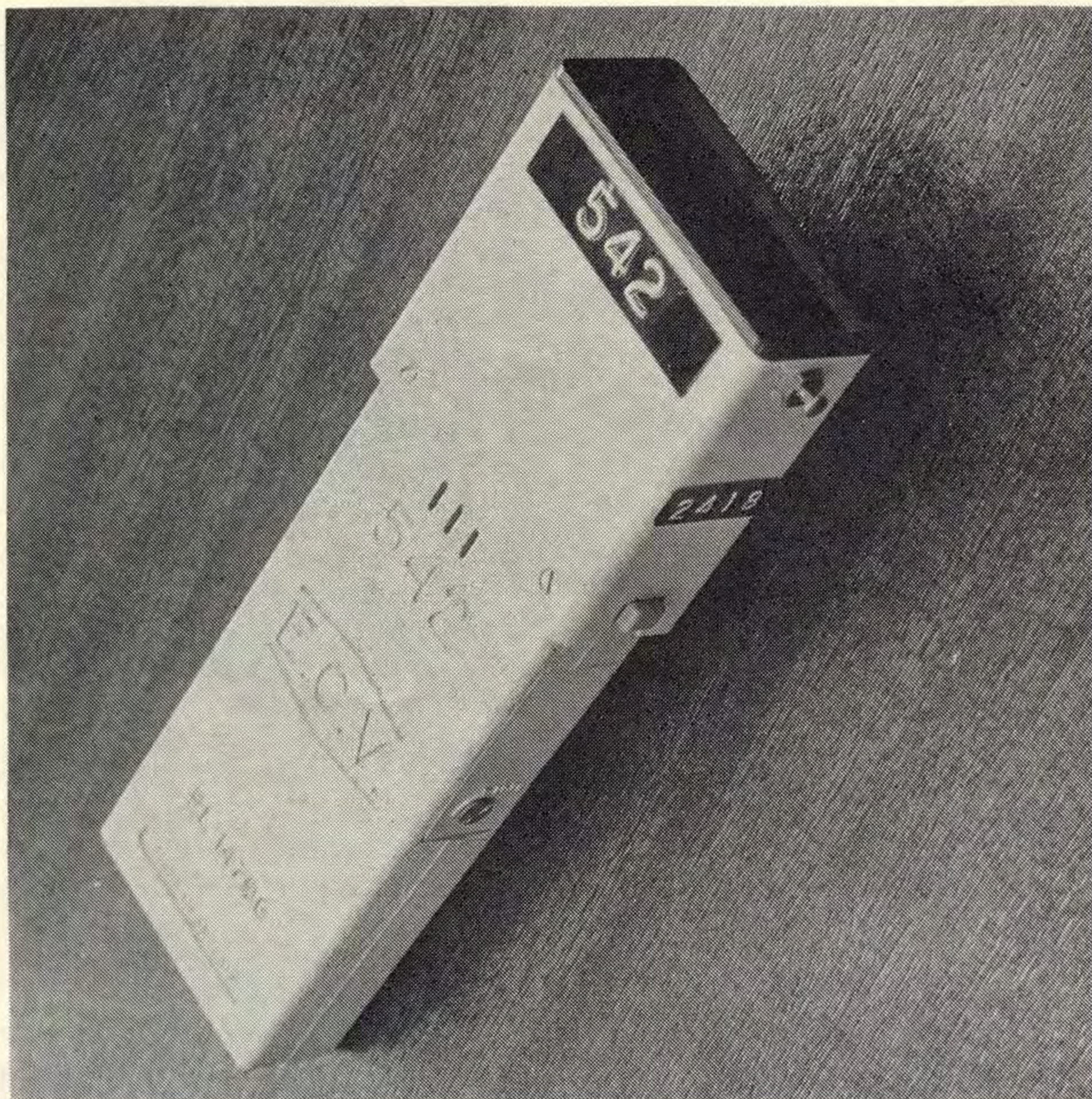
The pocket receiver gives out a two-tone call with different pulse cycle for ordinary and urgent calls.
