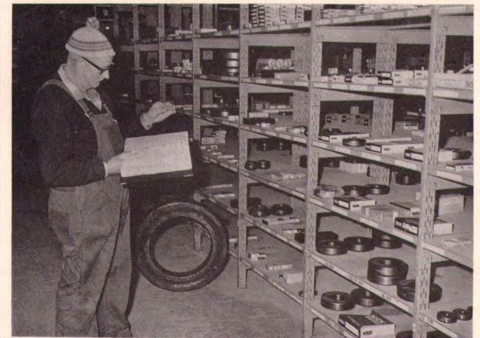
John Burke, a Storeman at Yallourn Stores, demonstrates the wide range of ball bearings held in stock. He is holding a \frac{3}{8} " (9.52 mm) O.D. and \frac{1}{8} " (3.175 mm) I. D. bearing, whilst the one on the floor has an O.D. of 25" (620 mm) and an I.D. of 16" (420 mm).
