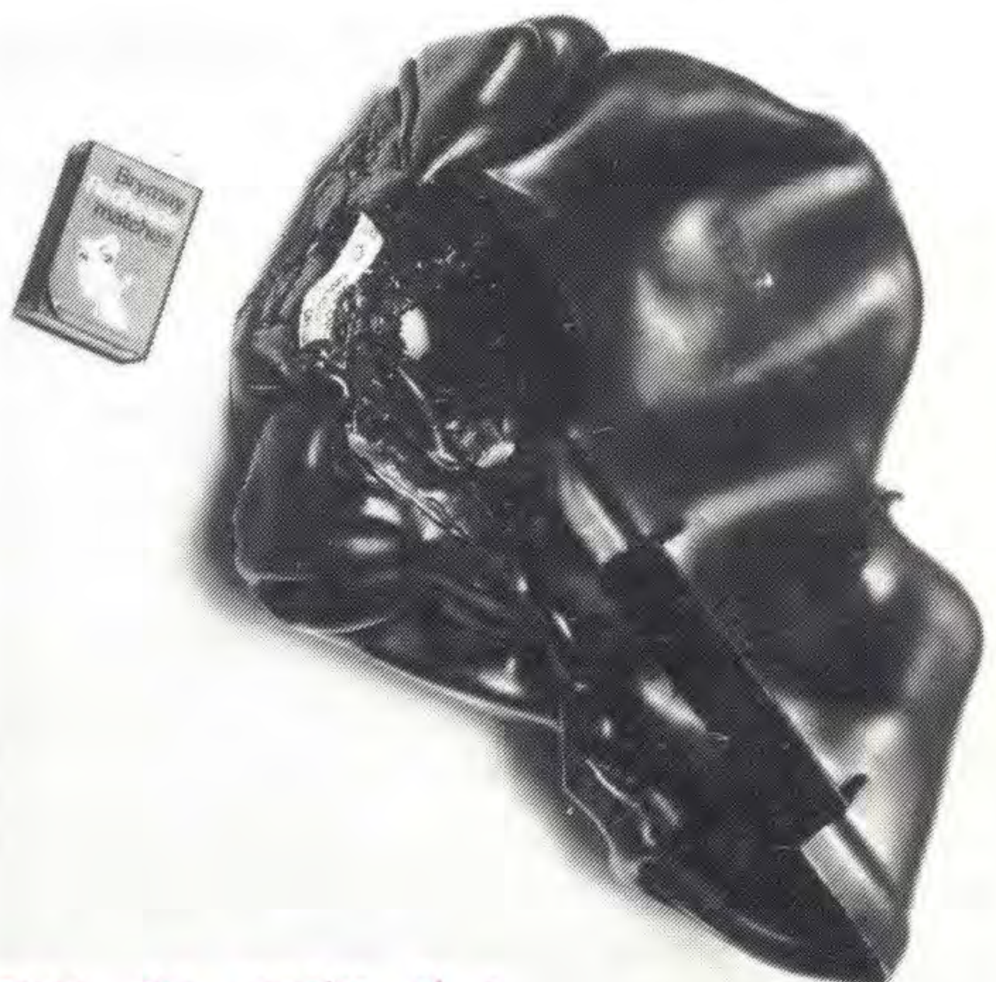
Right: The remains of a plastic bin after burning for only seven minutes.
