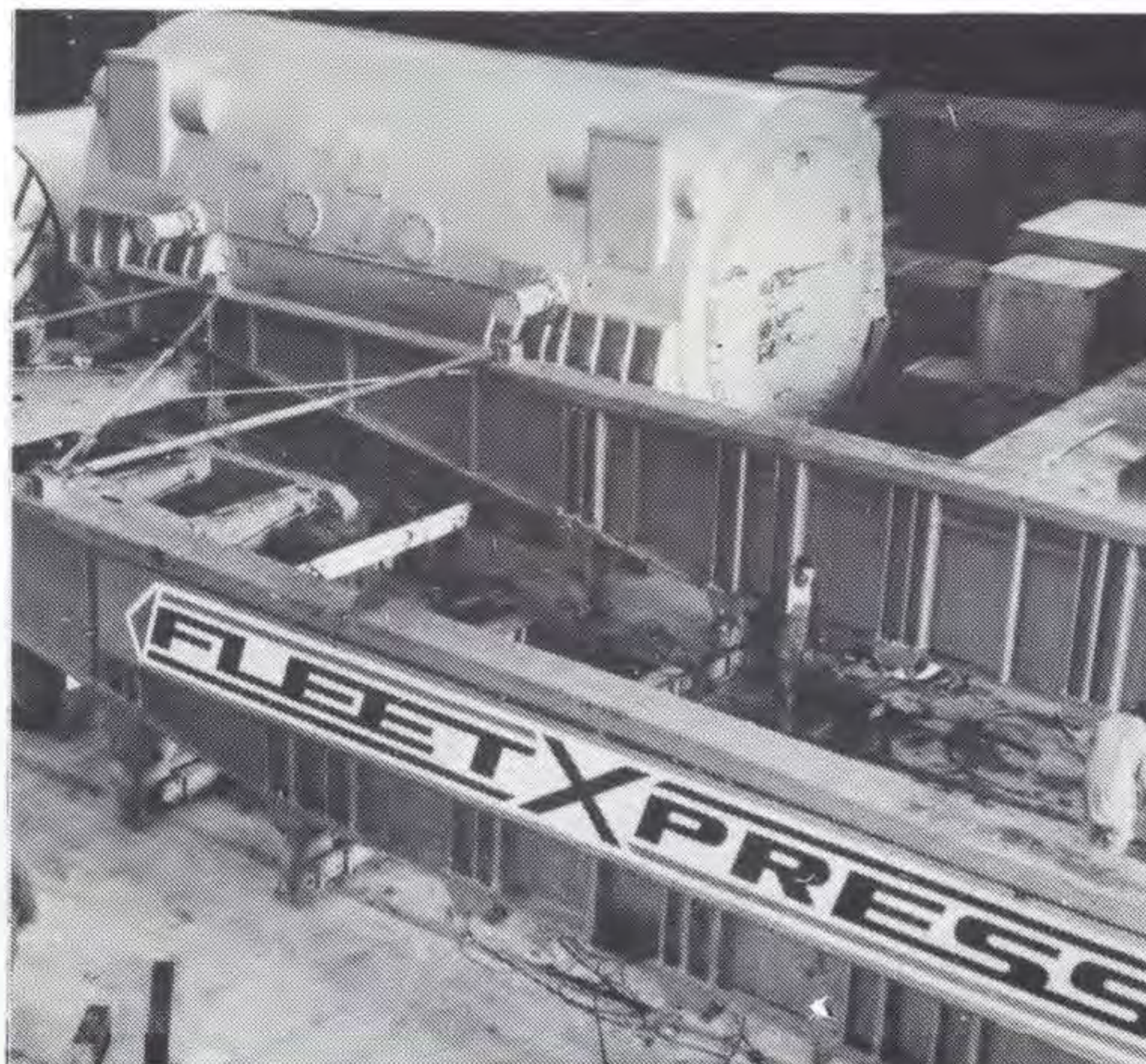
The large turbine casing is at the top of picture while the special Fleetpress lowloader is in the foreground.
