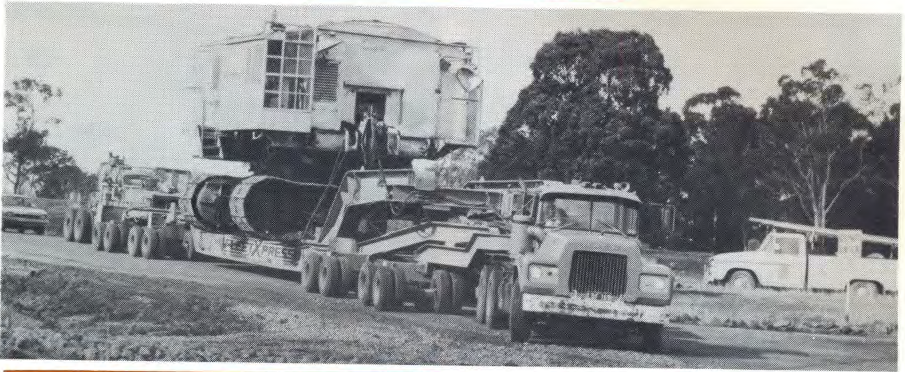
The large low loader carrying the dragline is pictured (above) about to enter the old Midland Highway.
