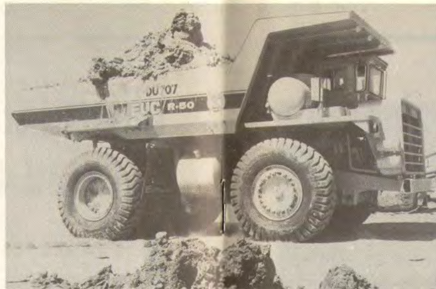
On its way to the overburden dump is a fully laden 50-tonne Euclid truck.
