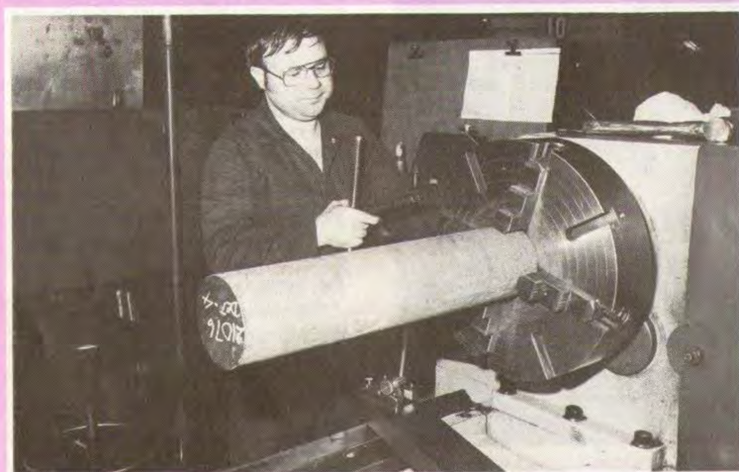
Fitter and turner Gennady Starikov sets a shaft in a lathe.
