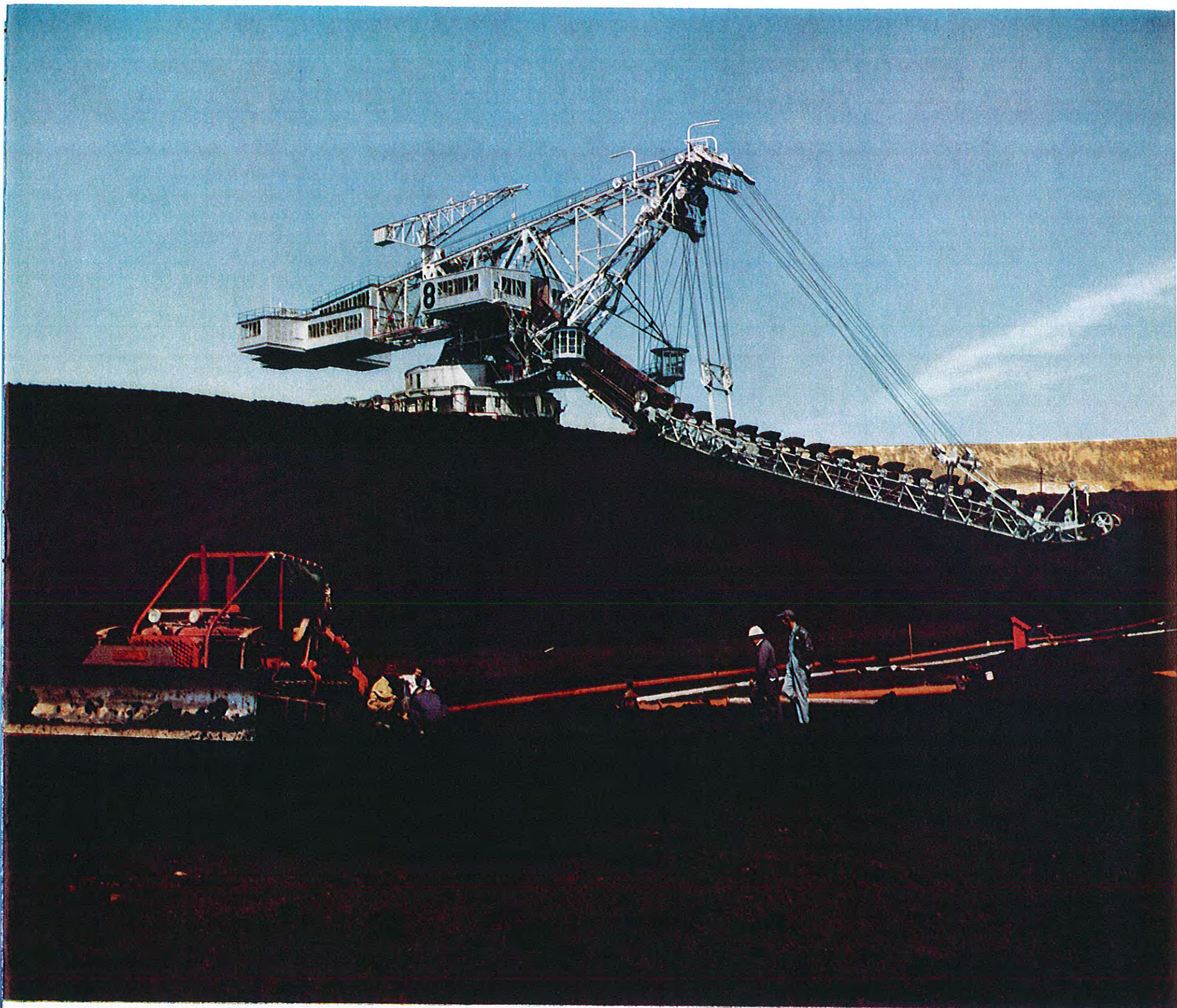
Bucket-chain coal dredger, Yallourn Open Cut
