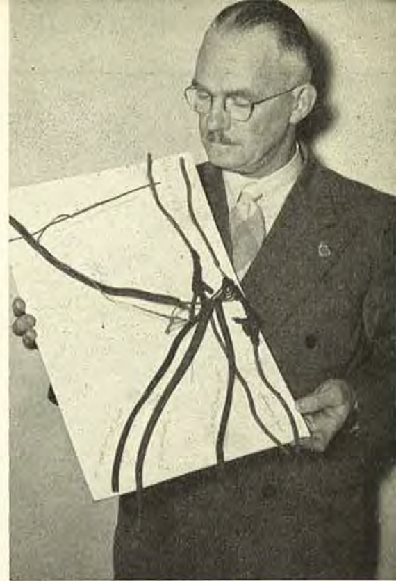
Mr. J. C. Malins, Investigation Officer, displays an example of dangerous work—bare wire, rough taping, useless earth, new lines tapped off original conductor.
