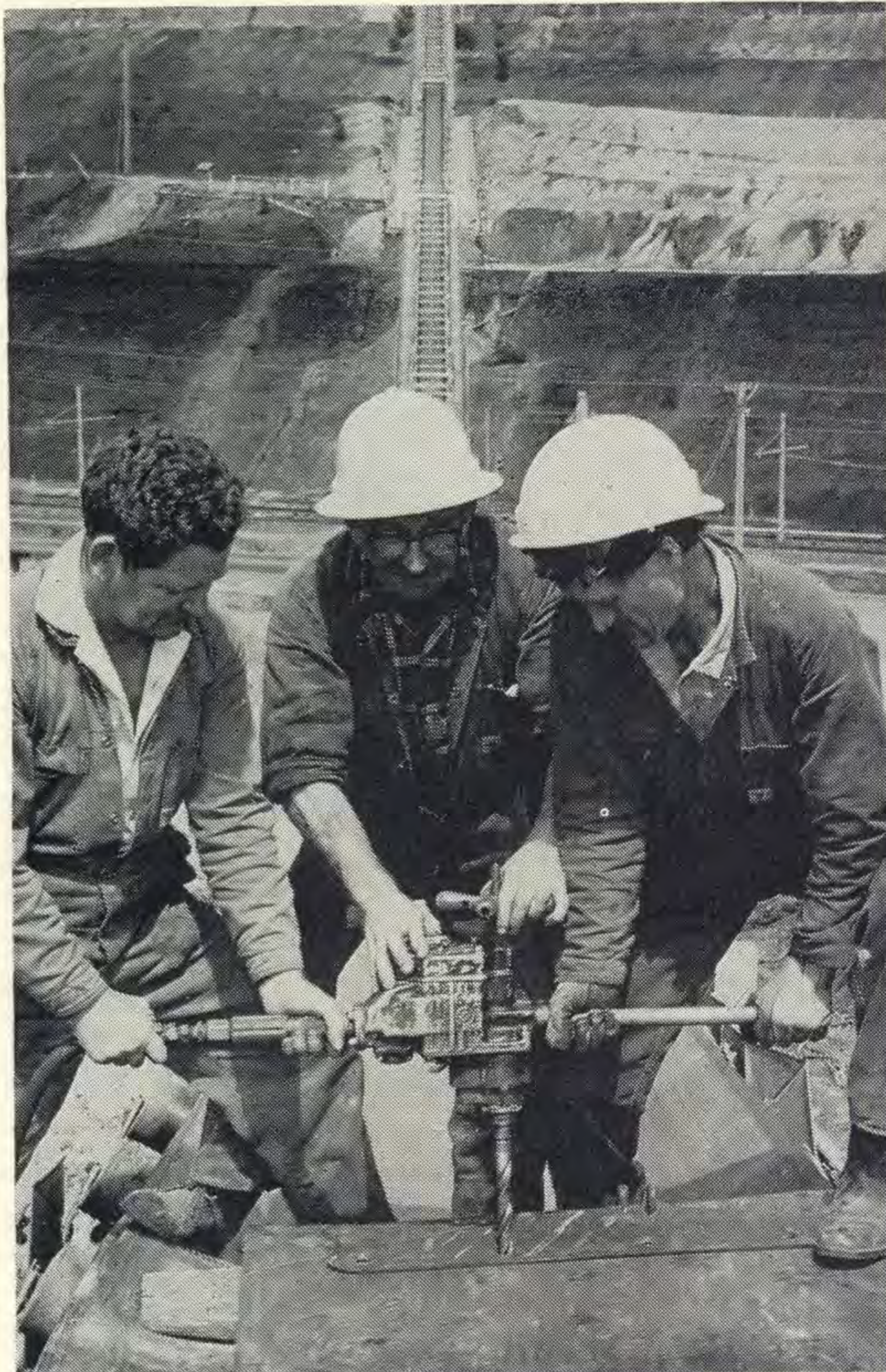
Frank Holt, Phil Sheekey and Lindsay Burns fit a towing attachment to the end of No. 11 conveyor belt ready to pull the belt up to the vulcanising position.
